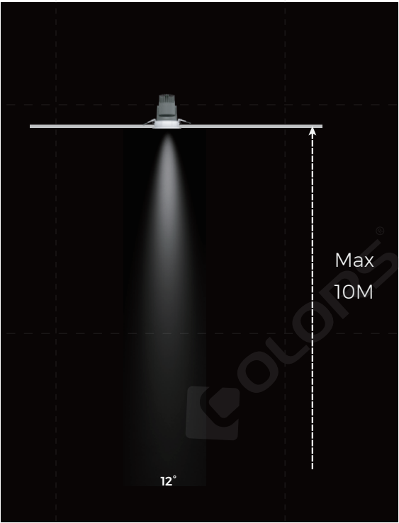
Ultra-Narrow Angle 12° Maximum Mounting Height 10m
