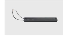
Magnetic power Model: MT20-HDRV200H48S-M Size: L305*W22.5*H46mm Input voltage: 220-240VAC Output: DC48V Power: 200W Applicable model: All straight track
