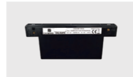
CASAMBI Control Model: 1200EN1812-CAS-W0-BLDAV48 Size: 142.6*18*58.1mm Input voltage: 48VDC Output signal: DALI Output DALI Max.current: 180mA Control devices: ≤64 Control groups: ≤8 Certification: CE, UKCA Others: Controller should be used with DALI dimming modules.
