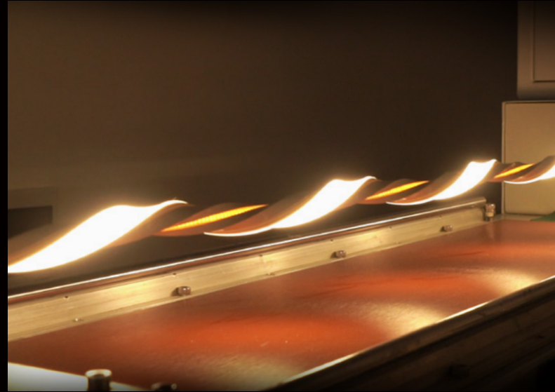
Twisting test * 720°*5000times
