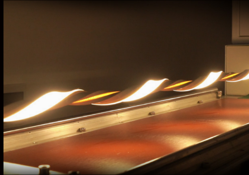
Twisting test * 720°*2000times
