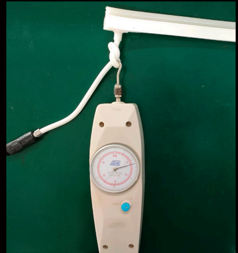
Tensile Test (for end cap): Four times neon weight
